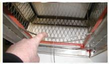
For cleaning, remove the cable guide support by pushing down hard enough so the cable guide support "pops" out of its mounting holes.
